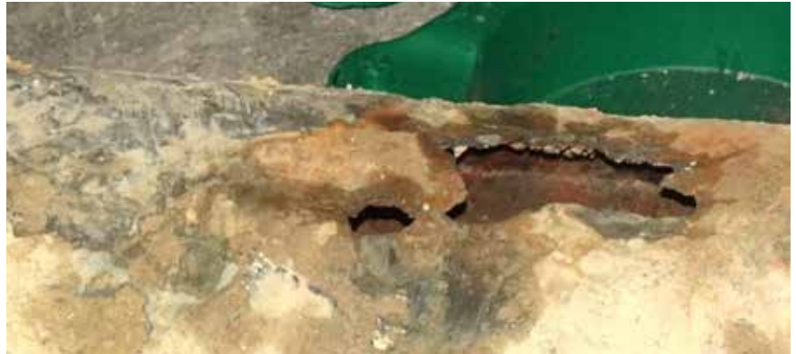
Corrosion of waterpipe made out of ductile cast iron.
